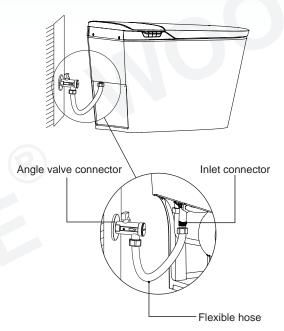
Connect the water inlet and angle valve of the toilet with the matching hose and tighten it
